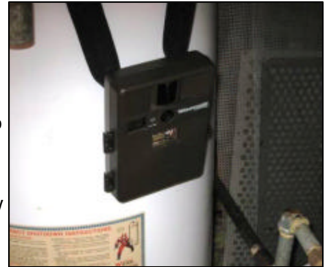
Test run of the motion-activated camera. The camera is mounted on a resident's home water heater.
