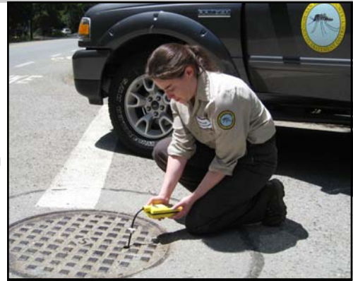
Theresa Shelton takes gas level readings on a typical sewage line access point.
