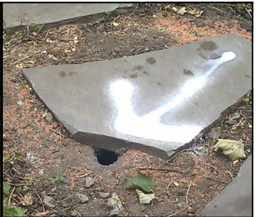
Locations were marked with arrows where smoke was observed escaping to the surface due to breaks in residential sewer lateral lines.
