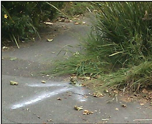
Locations were marked with arrows where smoke was observed escaping to the surface due to breaks in residential sewer lateral lines.
