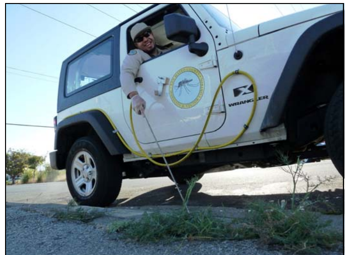
A team of seasonal technicians crisscrosses the county during the summer months to treat catch basins using specially-modified right-hand-drive jeeps.
